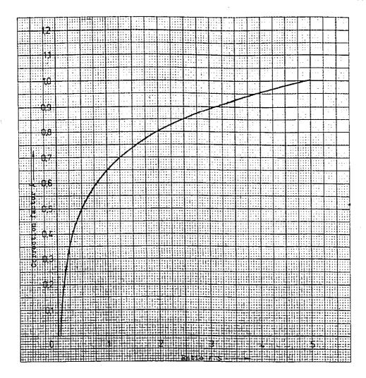
In the case that there are only small requirements for the determination of blanking lengths, the rounded values collected to groups according to Table 5 may be applied for the correction factor k.
