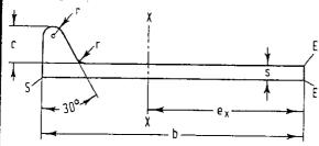
Designation of a hot rolled bulb flat (shape letters HP) of width b = 200 mm and thickness s = 10 mm, made of shipbuilding steel A according to the prescriptions of the Germanischer Llöyd (GL, see Section 4), material number 1.0441:
